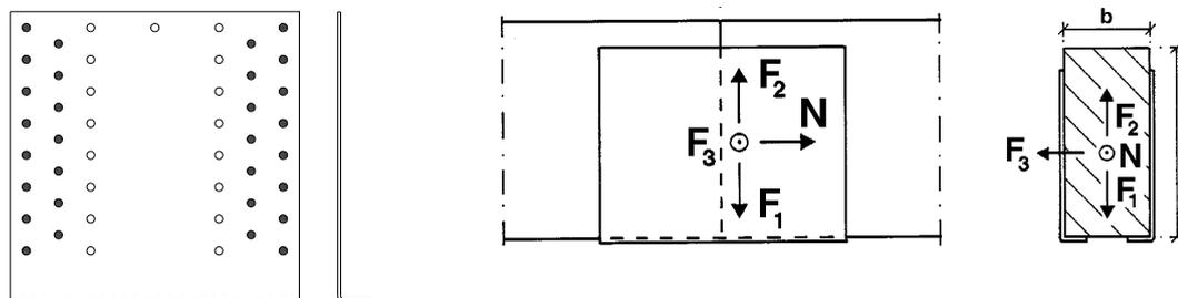
Nails in 2 end columns applicable for shear forces  $F$  combined with normal force  $N$
