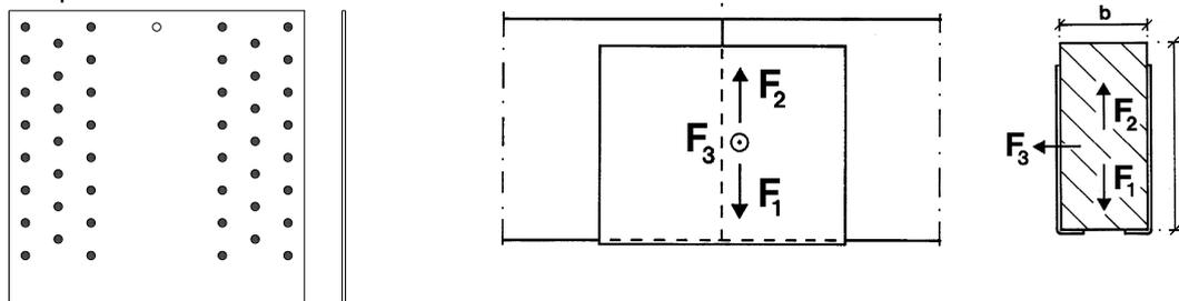
Nails in all holes applicable for shear forces  $F_1$ ,  $F_2$ ,  $F_3$  only.
