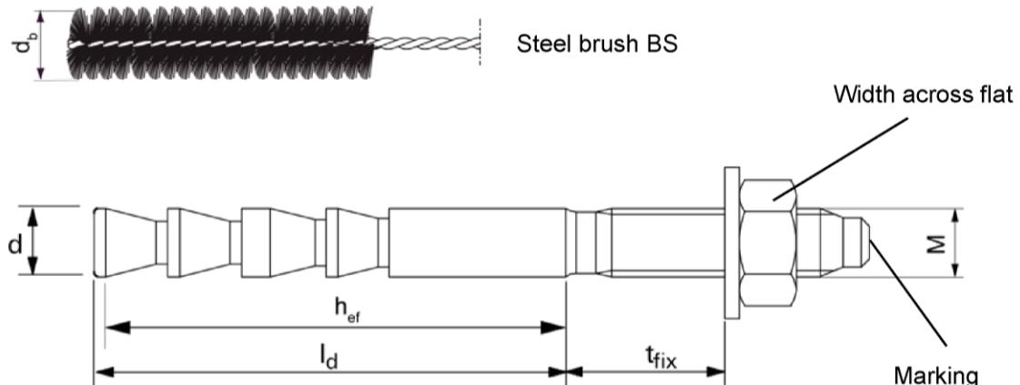
**Marking:** Work symbol; size, anchorage depth  $h_{ef}$ :
