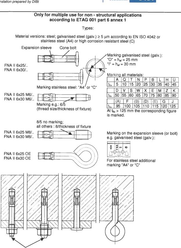
Additional marking only for galvanised steel (galv.) at effective anchorage depth  $h_{ef} \approx 25 \text{ mm}$ (centering, bar or point)
