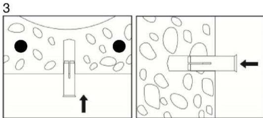
Fixing is not allowed for  $h_{ef} = 25 \text{ mm}$  and  $d_b < 35 \text{ mm}$  when a cavity is cut!
