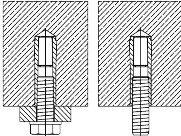
**Intended use in precast pre-stressed hollow concrete slabs ( $w/e \leq 4,2$ ) with a flange thickness  $\geq 35$  (or 30 mm  $\rightarrow$  see Annex C2) and only for  $h_{ef} = 25$  mm**
