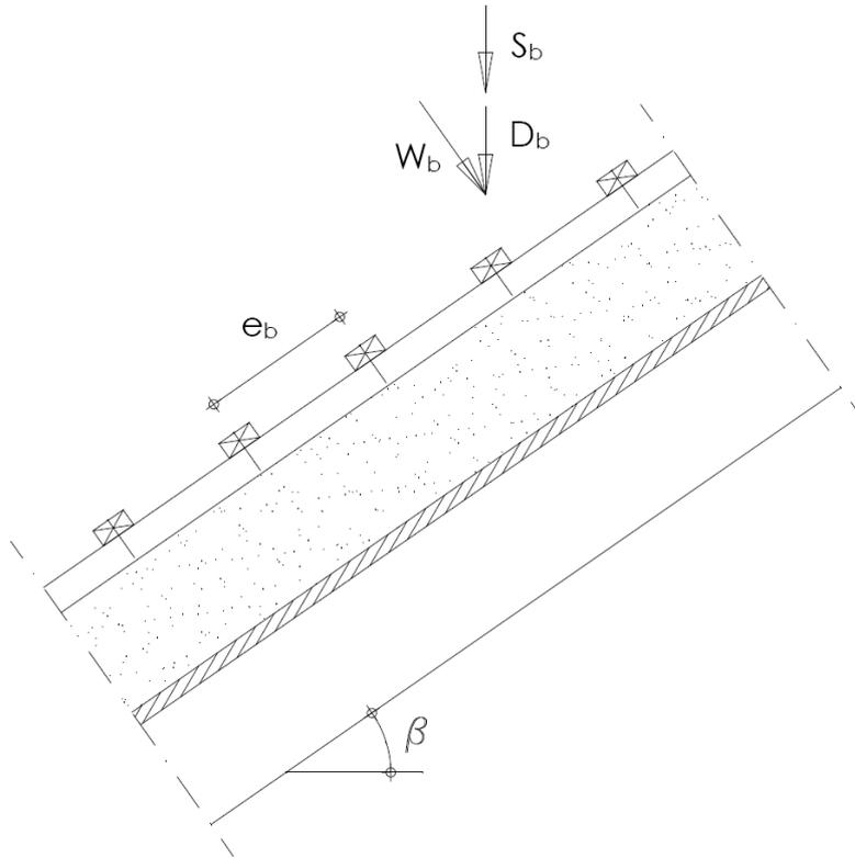
$$\begin{aligned} D_b &= d \cdot e_b \cdot e_r \\ S_b &= s \cdot e_b \cdot e_r \cdot \cos \beta \\ W_b &= w_p \cdot e_b \cdot e_r \\ F_b &= W_b + (D_b + S_b) \cdot \cos \beta \end{aligned}$$
