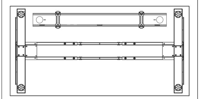
Put the cable tray click with the holders on the table top and screw holder brackets tight in the top.
