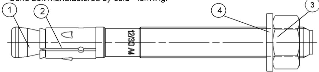
Cone bolt manufactured by turning:
