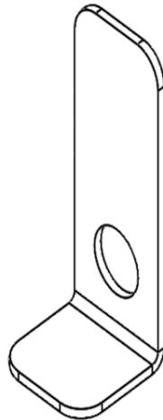
Sheet material with a thickness of 5 - 8 mm applicable.
