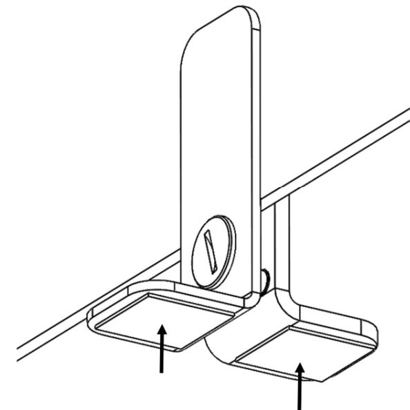
Remove the protective film from the adhesive pads.
