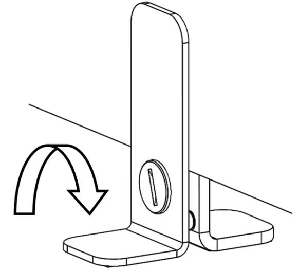
Tighten the screws on both brackets.
