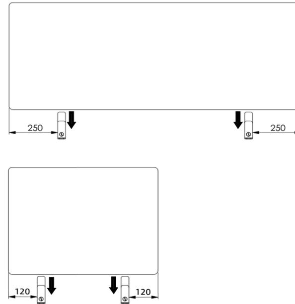
Position the brackets on the "screen". We recommend a distance of 120/250 mm.
