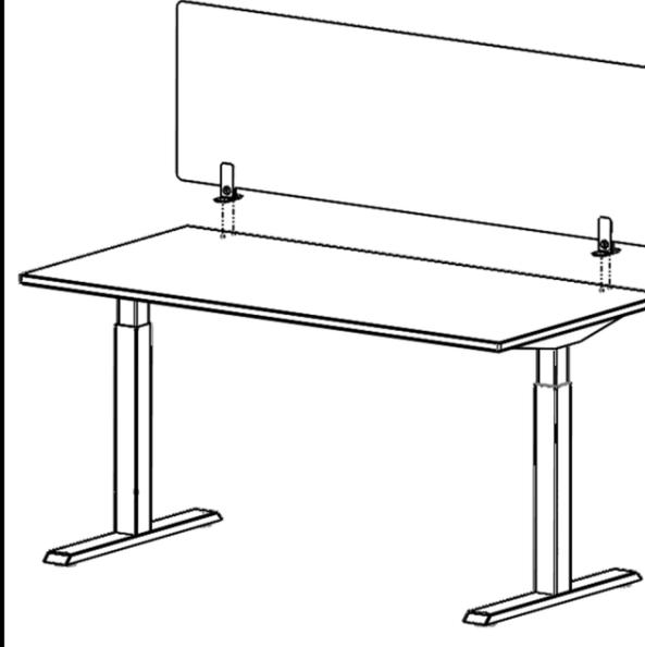
Degrease the adhesive surface before using the adhesive pads to the bottom.
