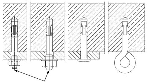
Additional marking only galvanised steel for h<sub>ef</sub> = 25 mm (centring, bar or points)
